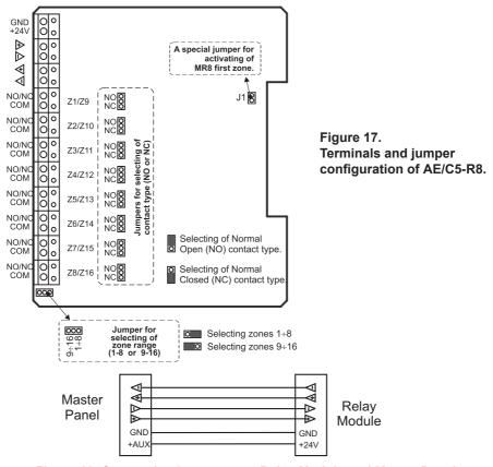
Figure 18. Connecting between one Relay Module and Master Panel.
